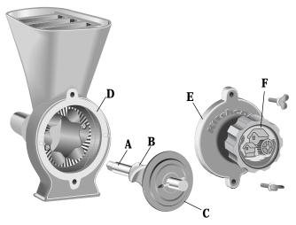
Insert the attachment power shaft (A) with the grind worm (B) and movable burr (C) into the grain mill body (D). Mount the front plate (E) with adjustment knob (F) onto the front of the shaft.
