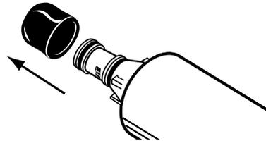
4. Slide the cartridge cap onto the new cartridge as shown.
